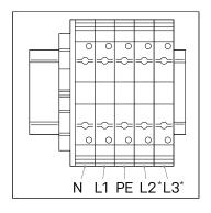
Attention: Do not connect the phase cables L1, L2 or L3 in the PE or N connectors.
