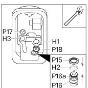
**Attention:** Ensure that grommets and the cable gland are inserted correctly, to quarantee resistance to ingress of water and dust.
