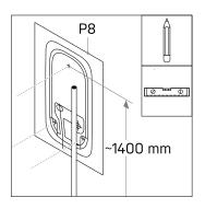
Mark and strip the mains cable at 10mm above the mains wire entrance as indicated on the template.
