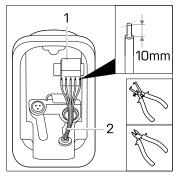
Attention: Ensure that the power cables are located right from the bracket (2).
