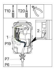
**Attention:** Connect the phases, neutral and protective earth with the correct connector in the cover. The correct order is indicated on the cover: PE - L3 - N - L2 - L1
